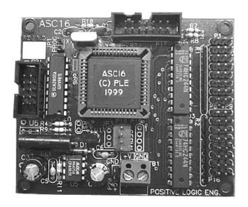
Figure 5.24: The ASC16 servo controller board<sup>19</sup>.
