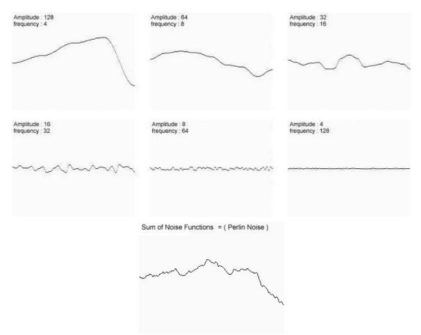
Figure 2.5: Perlin Noise The Perlin noise (the bottom signal) is the result of the sum of the six signals above it<sup>6</sup>.
