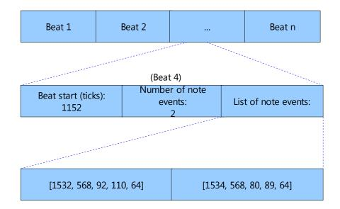
Figure 5.9: Structure of the output of Stage 1
