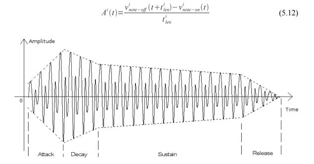
Figure 5.5: The looped sample from Figure 5.4 modulated with the ADSR envelope<sup>14</sup>.
