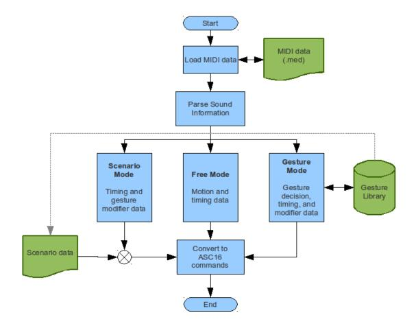
Figure 5.23: The complete system (Note: the Gesture Mode is not yet implemented but for future reference)
