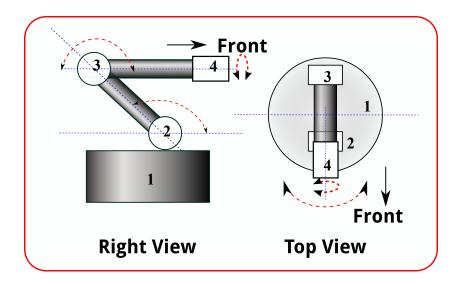
*Figure 5.17: Configuration of the custom Lynxmotion robot.*
