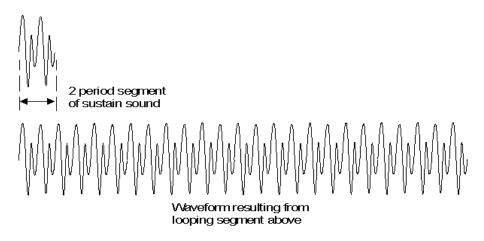
Figure 5.4: A sampled sound segment and the same segment looped<sup>13</sup>.
